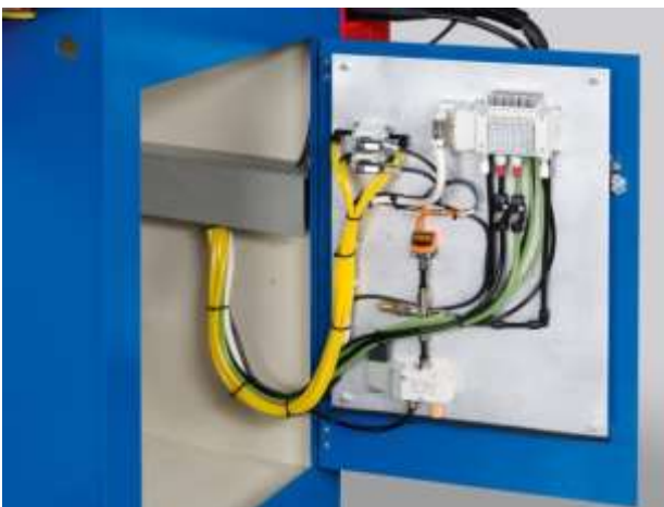
Figure 4: Pneumatics easily accessible from front of machine
