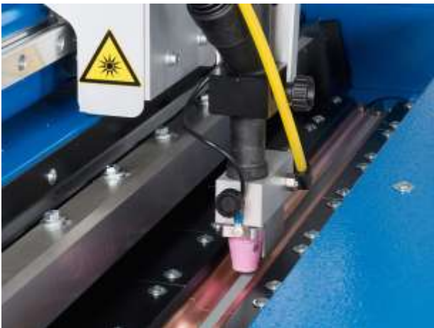
Figure 3: Clamping system, torch with trailing gas shield, centre stop on the left
